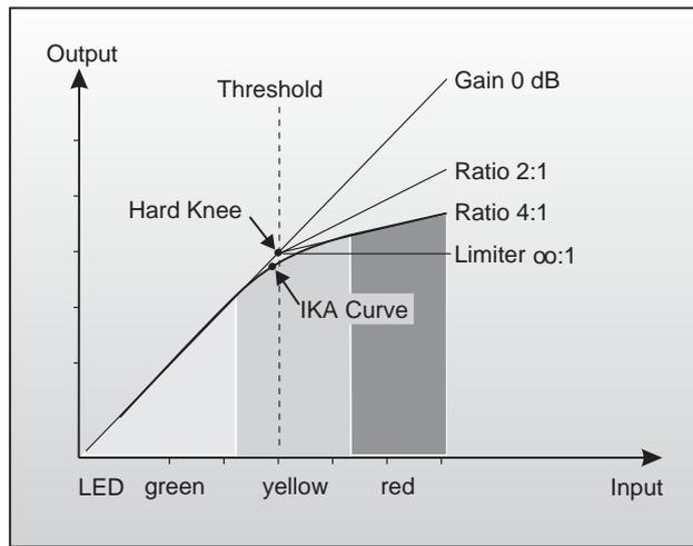
Fig. 4.2: IKA characteristic of the compressor section
