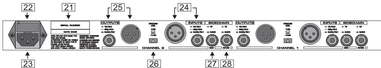
Fig. 2.5: Control elements of the rear panel
