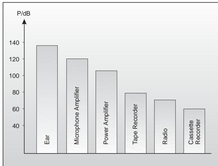
*Fig. 3.1: The dynamic range capabilities of various devices*
