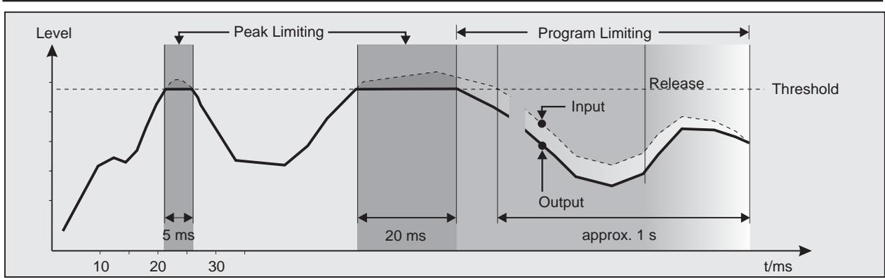
Fig. 4.3: IGC characteristic of the limiter section
