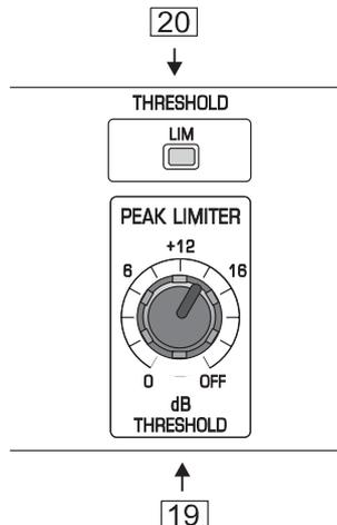
Fig. 2.4: Control elements of the peak limiter section
