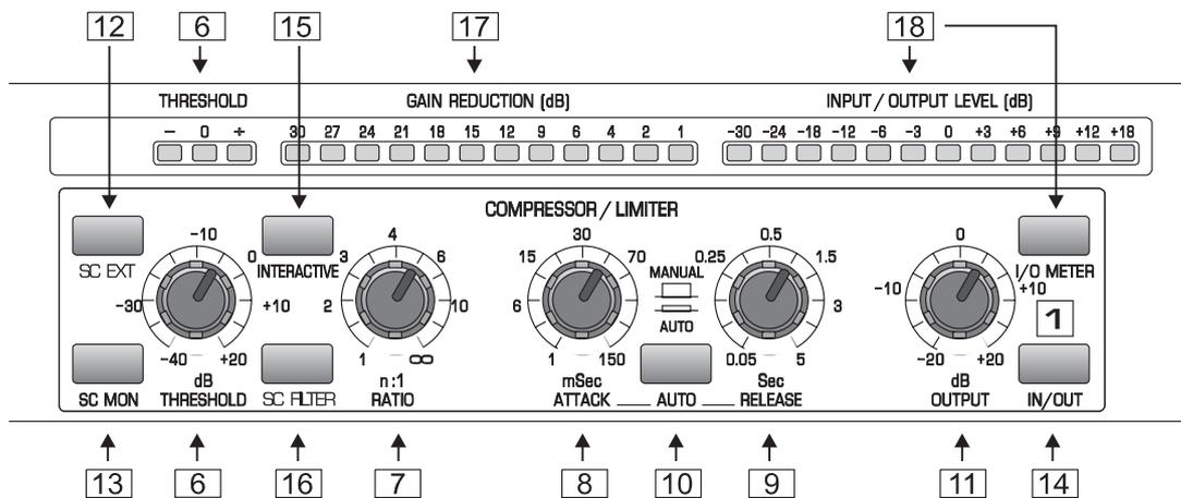
Fig. 2.3: Control elements of the compressor section
