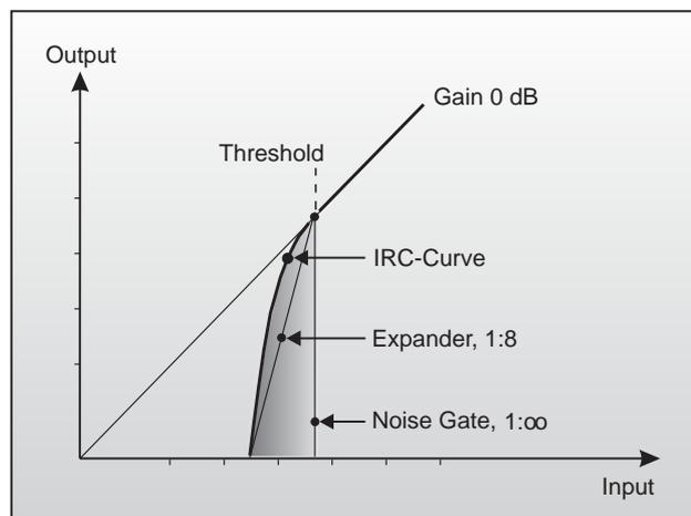
Fig. 4.1: IRC curve characteristic of the Expander
