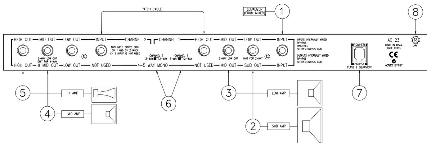
**Note:** The internal switching in the AC 23 will result in a Mono 4-Way configuration with the crossover sections arranged SUB, LOW, MID & HIGH from left to right across the front panel. By connecting a patch cable from the CHANNEL 1 HIGH OUT to the CHANNEL 2 INPUT, the LOW/MID crossover range changes from 70 Hz - 1 kHz to a higher range of 190 Hz - 7 kHz. Set the CHANNEL 1 switch to 3-WAY, and the CHANNEL 2 switch to 2-WAY.
