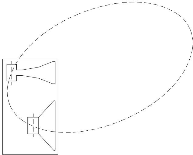
Fig. 1 In-Phase Axis Response Without Time Delay
